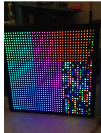
Figure 5: PCB Display with Distorted Signal
